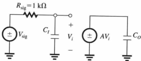
$$v_O = A v_i = A \cdot v_{\text{sig}} \frac{1/C_I s}{R_{\text{sig}} + \frac{1}{C_I \cdot s}}$$
